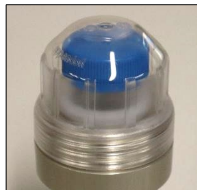
Figure 11. Aerosol cap attached to centrifuge bucket
