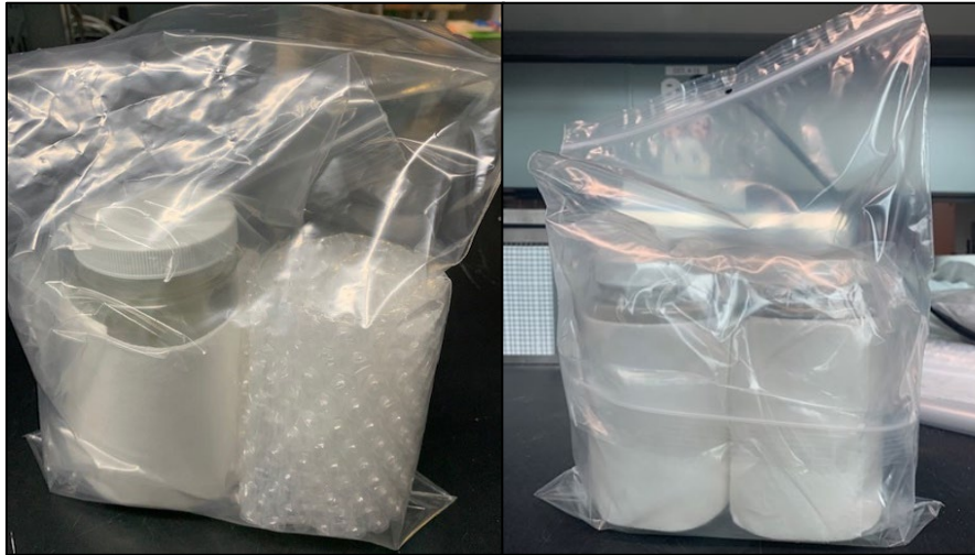
Figure 3. Double bagged single bottle and a buddy roll (left) and two bottles bagged (right)
