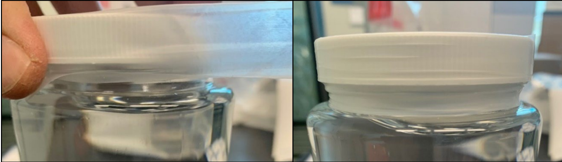
Figure 3. Stretching and applying the parafilm along the bottle lid
