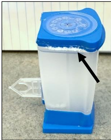
Figure 1. GeneXpert test cartridge, black arrow pointing to crystallization
