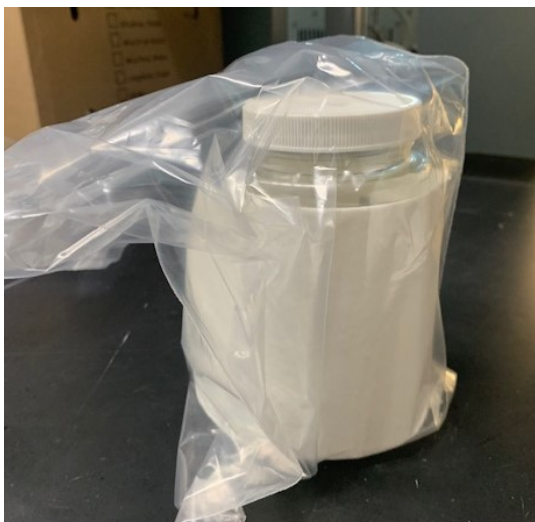
Figure 3&4 Examples of one and two bottles in primary re-sealable bag with absorbent
