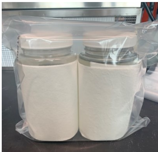
Figure 3&4 Examples of one and two bottles in primary re-sealable bag with absorbent
